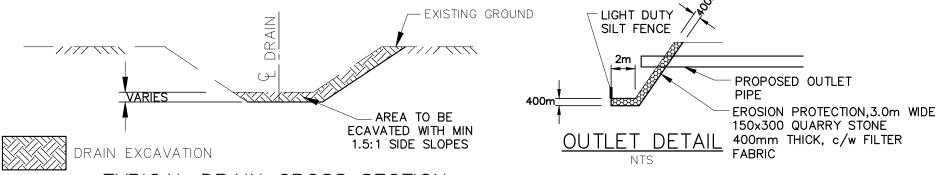
TYPICAL DRAIN CROSS SECTION
